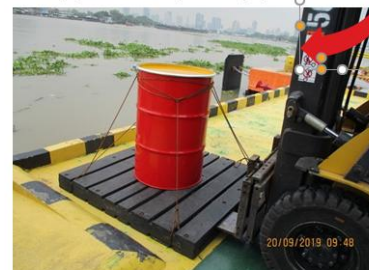
Tied equipment by ropes prior moved from the jetty front by forklift, then carried to storage area by pick-up truck
